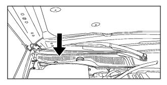
The access panel for the passenger compartment air filter is located under the hood near the windshield, on the passenger's side of the vehicle. See *Engine Compartment Overview on page 373* for more information on location. See *Doing Your Own Service Work on page 364* for information on doing your own service work.
